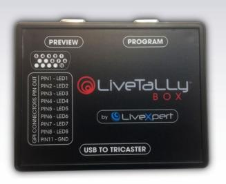
You can refer to the label to locate the pin from each connector.
